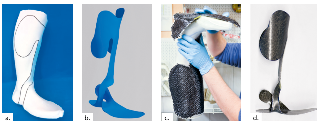
Fig. 5a–d Orthosis with a complex geometry – from digitised plaster model to finished component.
